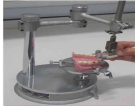
Figure 2: Paralleling device
